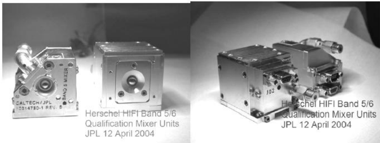
Figure 5: Qualification model band 5 and band 6 mixers
