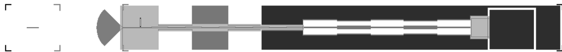
Figure 10. 350 GHz Junction layout. The radial probe antenna is visible on the left side. The IF is taken out via a microstrip RF choke (on 300 nm SiO, \epsilon_r=5.6 ) which connects to a high impedance CPW transmission line (inductive) and shunt capacitor. This LC mechanism provides a \pi tuning network with the combined capacitance of the Probe, twin junction RF tuning structure, and microstrip RF choke. The IF passband of mixers under discussion has been optimized to cover 1-13 GHz.
