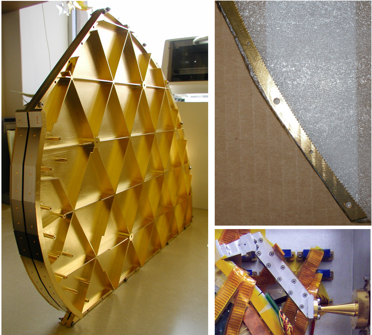
Figure 2. [Left] Z-Spec spectrometer assembled showing light-weighted rib structures. The input feed mounts on the top-most flat surface and bend blocks mount on the other eight flat surfaces. The longest dimension in the structure is 55 cm. [Top Right] View of small segment of the grating. [Bottom Right] Corrugated feed horn for coupling to the telescope, waveguide taper, and input feed which illuminates the grating.
