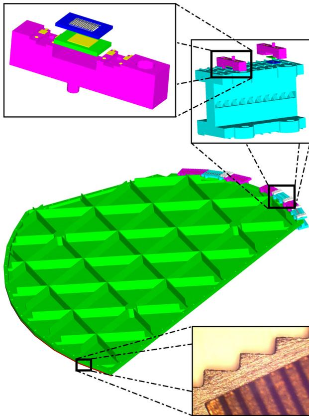
**Figure 2:** The grating is shown in the center with light-weighting on the exterior visible. The lower right panel is a photograph of the prototype blazed surface. Each facet (cut by wire EDM) is approximately 1 mm wide. Above and to the right is a schematic drawing of a mitred waveguide bend block. Radiation enters along the middle and is reflected up and down alternately in adjacent channels. The upper-left drawing is a single bolometer module with a backshort and bolometer shown.
