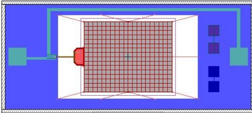
**Figure 5:** Z-Spec bolometer mask. The  $\text{Si}_3\text{N}_4$  absorbing mesh is in the center; the filling factor of the grid is a few percent. The square wirebond pads that are vapor deposited on the  $\text{Si}_3\text{N}_4$  top layer of the wafer can be seen on the left and right.
