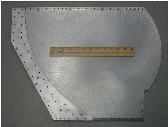
**Figure 3:** Z-Spec prototype grating with one plate removed. The blazed surface is on the left. Assembled, the grating is 56 cm  $\times$  42 cm  $\times$  2.25 cm. A 12-inch ruler is shown for scale. The input horn is attached on the lower right, just below the curved focal arc. The output feed can be attached anywhere along the arc on the right side of the plate. Lower frequencies are focused close to the input horn, with higher frequencies arriving higher along the curve.
