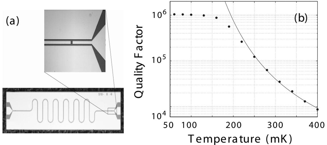
Figure 3: (a; left): Photograph of a CPW test resonator. (b; right): The measured quality factor  $Q = \nu_0/\Delta\nu$  as a function of temperature for an aluminum CPW resonator on a sapphire substrate.
