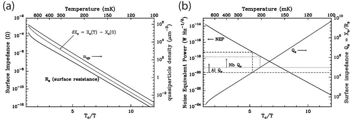
Figure 2: (a; left): The variation of  $\delta X_s = X_s(T) - X_s(0)$  with temperature follows the same exponential behavior as  $R_s$  and  $n_{qp}$ . (b; right): The surface impedance quality factor  $Q_s = X_s/R_s$  and the generation–recombination limit for the noise equivalent power (NEP) for a detector volume  $V = 10^4 \mu\text{m}^3$ , appropriate for bare pixel detectors.
