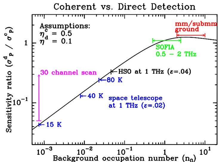
Figure 2: An idealized comparison of the relative sensitivities of coherent and direct detection. The vertical axis is the sensitivity ratio; a ratio less than unity favors direct detection. The vertical arrow shows the sensitivity penalty associated with a 30-channel sequential spectral scan.
