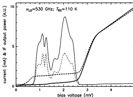
Figure 5: Measurement of a 530 GHz SIS mixer using a Nb/AlN/Nb SIS junction.<sup>8</sup> The unpumped current-voltage (IV) is the lowest solid line; the dashed curve just above is the pumped I-V curve. The double-peaked curves show the IF response to hot (295 K) and cold (80 K) blackbody loads. For this example, the sensitivity is a factor of  $\sim 10$  above the quantum limit.
