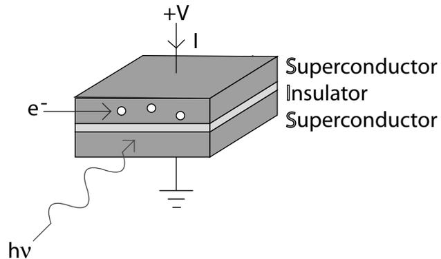
Figure 4: A superconducting (SIS) tunnel junction. Junctions are made from a Superconductor/Insulator/Superconductor trilayer, or SIS. A typical junction area is  $\sim 1 \mu\text{m}^2$ . Submillimeter photons are coupled to the junction via leads attached to the electrodes.
