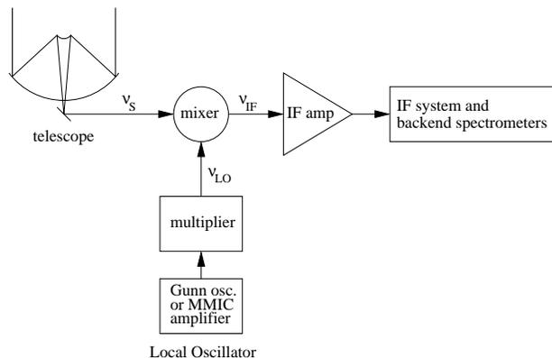
Figure 1: Block diagram of a heterodyne spectrometer. The telescope signal  $\nu_S$  is combined with a local oscillator  $\nu_{LO}$  in a mixer, to yield the intermediate frequency  $\nu_{IF} = |\nu_S - \nu_{LO}|$ .
