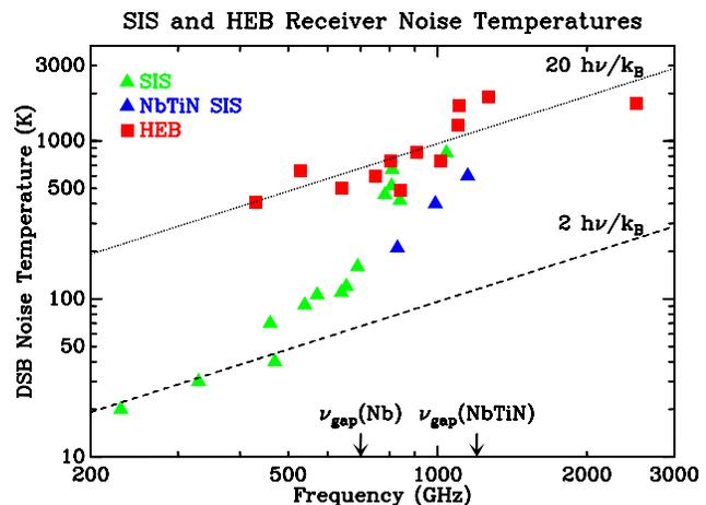
Figure 3: A selection of measured sensitivities for SIS and HEB receivers.
