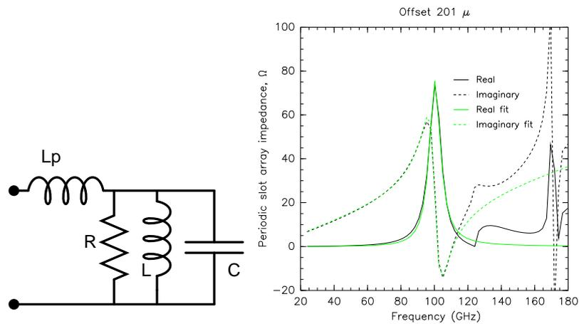
**FIGURE 5.** Equivalent circuit. Resistance  $R$  simulates radiation into dielectric and air. This circuit fits antenna impedance to a few percent in region of interest.
