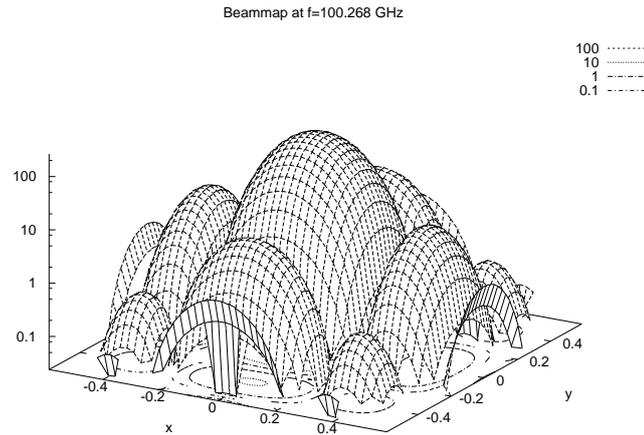
**FIGURE 3.** 15 by 16 antenna array beamshape vs.  $\sin(\Theta)$ . Array period is 700 microns, slot length 550 micron, offset 228 micron. The nearest sidelobes are at level of about 2.5 percent of central peak.
