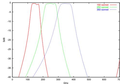
**FIGURE 2.** Transmission of three filters with bandpasses centered at 150, 250 and 350 GHz. Because of small (compared to wavelength) size of filter elements, the next resonance of 150 GHz filter does not start until well beyond the range of highest frequency filter, where it can be easily suppressed by lowpass filter if necessary.
