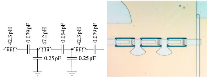
**FIGURE 1.** Filter schematics. Center frequency is 100 GHz, transmission line impedance – 5  $\Omega$ . On the right: 350GHz band filter manufactured at Micro Devices Laboratory (MDL) at JPL.
