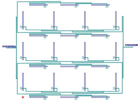
**FIGURE 4.** A small “baby” 4 by 3 dual polarizations array. It is shown for illustration purposes only. Dimensions are not to scale to avoid putting extremely fine details in a plot. The analyzed array has 15 by 16 antennas for each polarization. Stub capacitors impedance is used to tune inductive antenna to microstrip feed.
