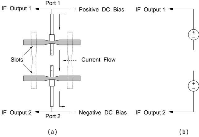
Fig. 3. Schematic showing how the two IF outputs for a given polarization are  $180^\circ$  out of phase: (a) shows the current flow for biasing the junctions in series and (b) shows the equivalent circuit.
