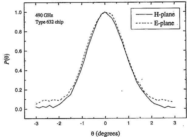
FIG. 4. The antenna profile of the quasioptical receiver measured along the  $H$ -plane (solid line) and  $E$ -plane (dash line). The  $-10\ \text{dB}$  width of the main beam is  $3.0^\circ$  along both directions. Sidelobes are slightly higher along the  $E$ -plane.
