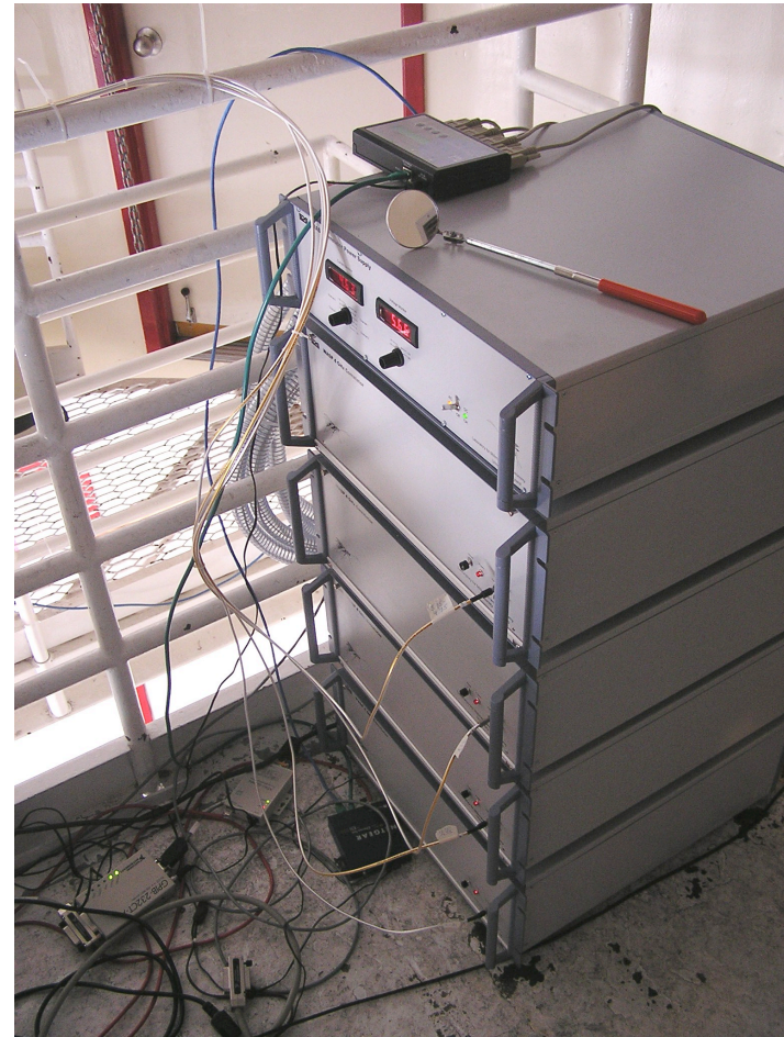
WASP II: 4 × 3.5 GHz analog correlator Andy Harris, U Md Future: sideband separating receiver with wideband digital backend
