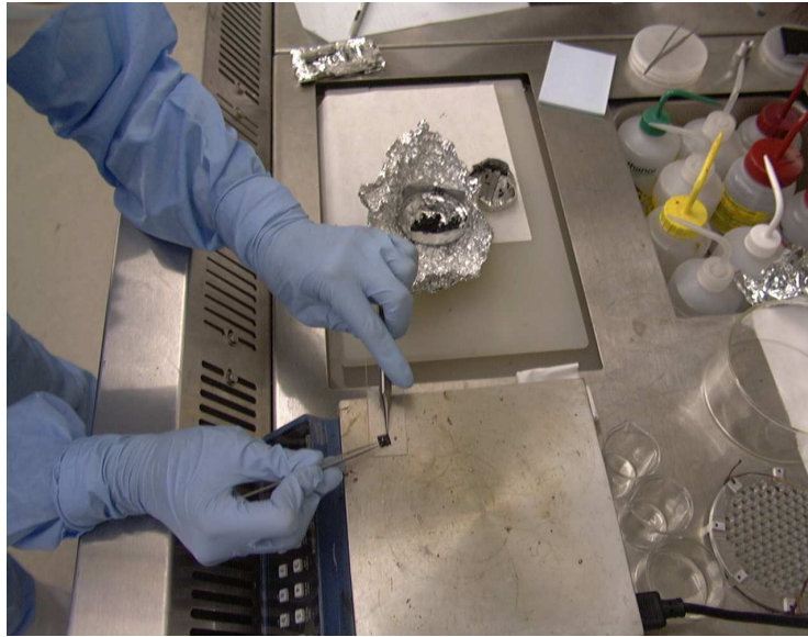
Figure A.12: The whole device must be protected before etching out the ‘window’ of silicon that defines the open area under the silicon nitride membrane. Here I am melting wax on the top side of the device.
