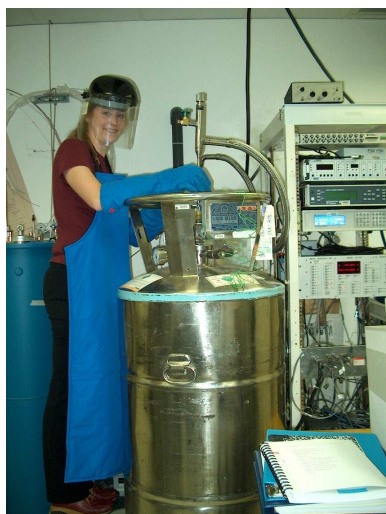
Figure 3.7: Filling the dewar with liquid helium.
