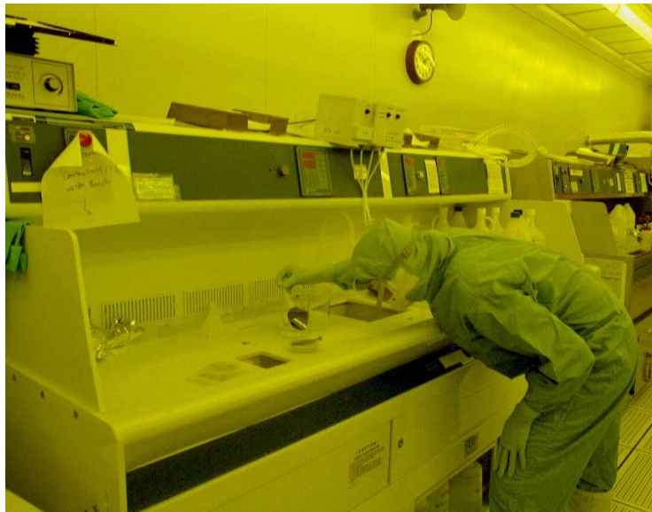
Figure A.9: ...the wafer is placed in a developer for a precise amount of time. In our 'positive' resist example, the developer washes away the broken polymer areas, leaving the pattern behind.
