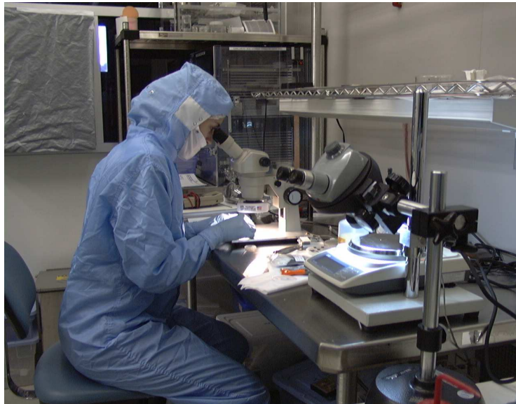
Figure A.11: For detectors with neutron transmutation doped germanium thermistors, the chips must be placed and bonded by hand. It can be a very time-consuming and tedious process.
