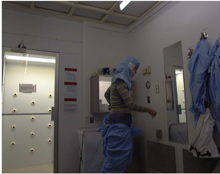
Figure A.2: Although you might be working in the class 1000 area, it is mandatory to satisfy class 10 gowning requirements since all areas are interconnected. Most of the gear we don is not to protect us from the chemicals we will use, but to protect our devices from us! Particulates can ruin a delicate device and make it difficult to work with.
