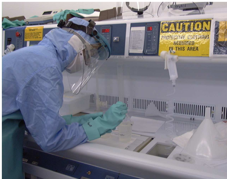
Figure A.14: The silicon window is etched from the backside either in a dry plasma etch process, or as shown here with hydrofluoric acid and nitric acid. After this step, the wax is dissolved in solvents and the delicate device is removed from the liquid, taking care not to break the membrane.
