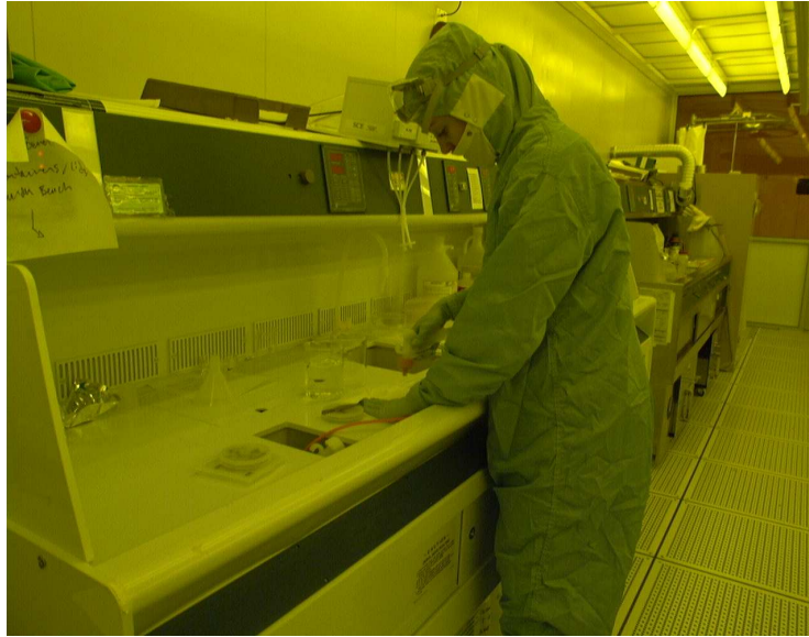
Figure A.10: The wafer has to be carefully dried before continuing the process. After this, the materials in the exposed areas are removed either in a wet etch or in a plasma etch, leaving behind a pattern under the photoresist. Finally the photoresist is removed in a solvent.
