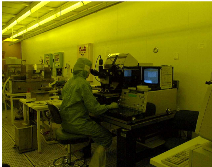
Figure A.7: A mask is used to create the desired pattern. The mask and wafer are placed in an aligner system. Once the proper placement is achieved, the wafer is exposed with the proper wavelength radiation for a set amount of time.
