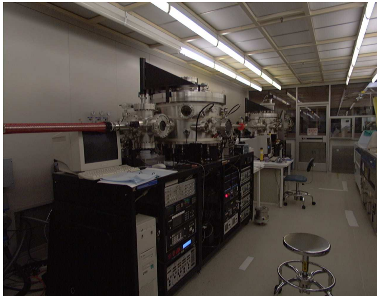
Figure A.5: Other materials, such as niobium, can be deposited in this sputtering system.
