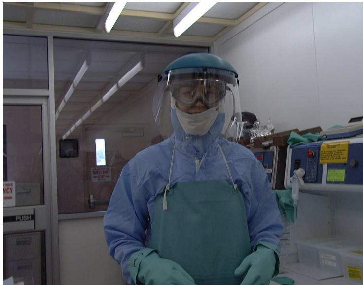
Figure A.13: Safety first! This is the personal protective equipment donned when handling acids. Besides the goggles, a faceshield, apron, and acid resistant gloves complete the ensemble.
