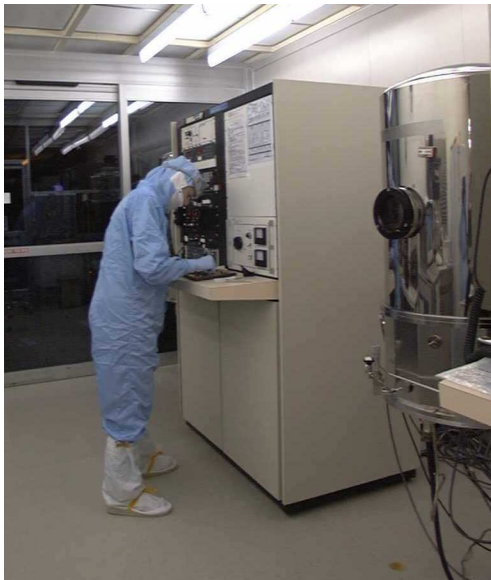
Figure A.3: The next few figures will show an example of a process layer. Here is an electron-beam evaporator, which can deposit various materials with relatively low impurity rates. In an etch-back process, the layer (such as gold) will first be evaporated at the appropriate thickness onto a silicon wafer.
