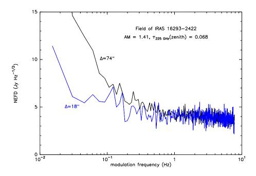
Figure 10. Observed NEFD for SHARC II at 350  $\mu$ m for a scanned observing mode without chopping. The 1/f noise is lower for pixels separated by 18" (bottom trace) than it is for pixels separated by 74" (top trace), which we attribute to variable gradients in sky emission.
