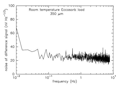
Figure 7. Noise spectrum for SHARC II observing room temperature Eccosorb foam. Even though shielding the foam from air currents significantly reduces correlated low-frequency noise over the array that we interpret as temperature drifts of the Eccosorb, there are still residual drifts with shielding. We show the power spectral density of the difference of two bolometer signals to subtract the residual correlated noise.
