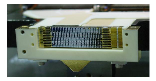
Figure 1. The SHARC II focal plane near the end of the assembly process. The bolometers cover an area of  $32 \text{ mm} \times 12 \text{ mm}$ .
