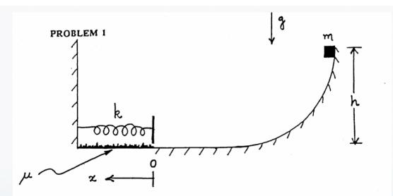
A block of mass m starts at rest and slides down a frictionless circular ramp from a height h. At the bottom, it hits a massless spring with spring constant k and in addition begins to experience a frictional force. The coefficient of kinetic friction is given by  $\mu$ .
