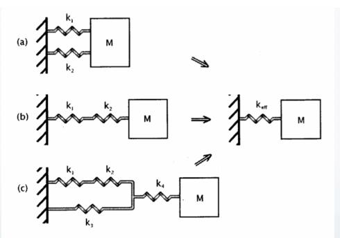
The restoring force on a spring is governed by Hooke's Law, F = -kx. Springs are linear devices, so any combination of springs can be modelled as a single spring with an effective spring constant  $F = -k_{\text{eff}}x$ . Refer to the diagram for parts (a), (b), and (c). Your final answers will not depend on M.
