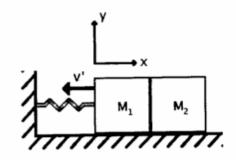
A second mass  $m_2$  comes sliding in with velocity  $-v\,\hat{x}$ , hits the first mass  $m_1$  at time t=0, and sticks to it. This induces oscillations in the spring, which can then be measured. This in turn can be used to determine the mass  $m_2$  of the impinging object.
