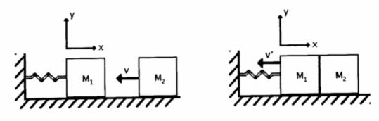
A second mass  $m_2$  comes sliding in with velocity  $-v\,\hat{x}$ , hits the first mass  $m_1$  at time t=0, and sticks to it. This induces oscillations in the spring, which can then be measured. This in turn can be used to determine the mass  $m_2$  of the impinging object.
