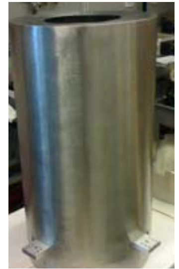
2-layer A4K mag shield < 1 mJy/degree mag signal
