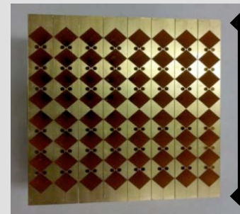
Stacked 1x8 Linear Arrays @ 350 GHz
