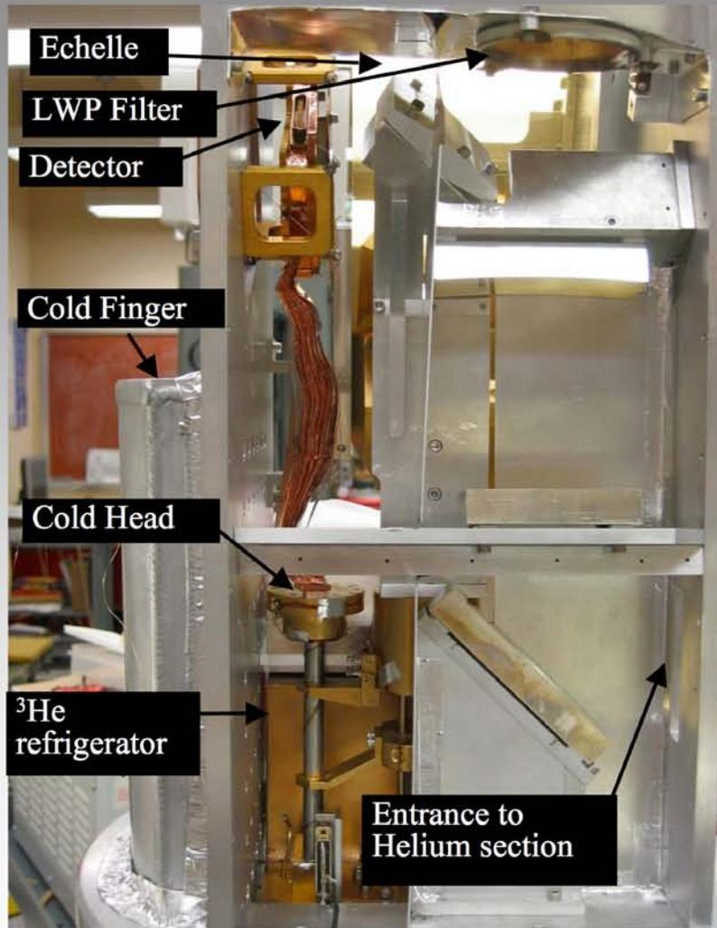
Interior of ZEUS with some baffles removed. The collimating mirror is hidden behind the middle wall baffles.
