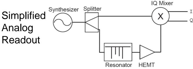
Software Radio for multiple channel readout
