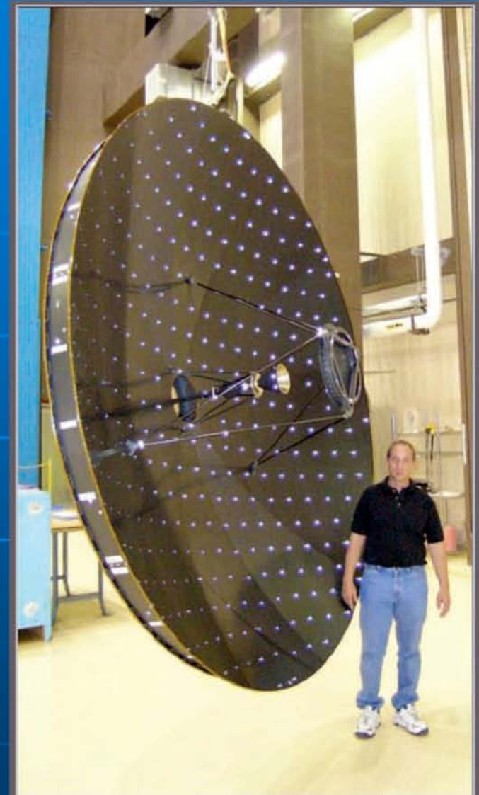
3.0-meter High Gain Antenna with 0.5-meter Sub Reflector
