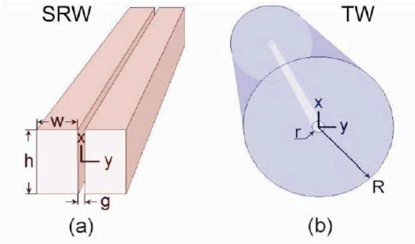
Fig. 1. Geometries of the considered dielectric waveguide structures: (a) A split rectangular waveguide and (b) a tube waveguide.
