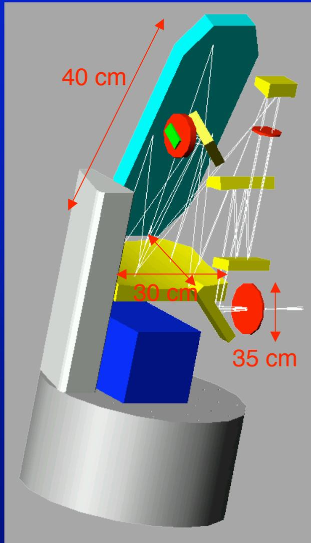
So grating and collimator are a large fraction of 1 meter in all dimensions -- 1.5-2 times larger than ZEUS
