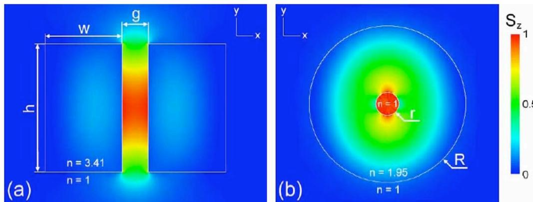
Fig. 2. Distribution of the normalized scalar  $z$ -component of the time-averaged Poynting vector  $S_z$  over a linear color scale in the cross section area of the waveguides. (a) Float-zone silicon split rectangular waveguide at  $f = 0.7$  THz with  $w = 54 \mu\text{m}$ ,  $h = 90 \mu\text{m}$  and  $g = 18 \mu\text{m}$ . (b) Fused silica tube waveguide at  $f = 0.5$  THz with  $R = 181.5 \mu\text{m}$  and  $r = 27 \mu\text{m}$ .
