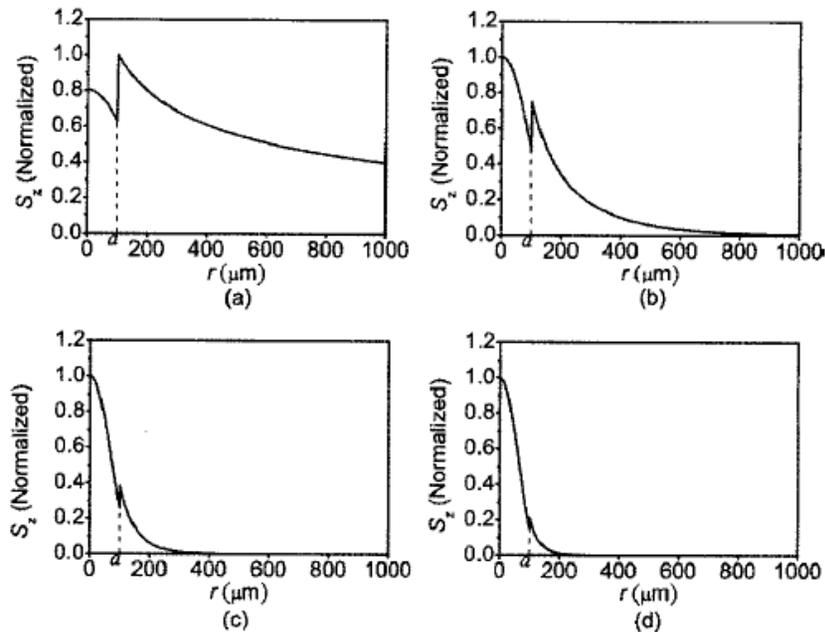
Fig. 1. Spatial distribution of the  $z$ -direction Poynting vector about a  $200 \mu\text{m}$  diameter ( $a=100 \mu\text{m}$ ) PE wire at frequencies of (a) 300, (b) 500, (c) 700, and (d) 900 GHz. The PE wire is assumed to be surrounded with air.
