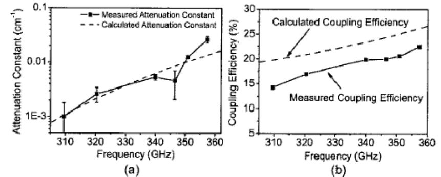
Fig. 2. (a) Measured fiber attenuation constant of the  $200 \mu\text{m}$  diameter PE wire in the frequency range 310–360 GHz. For comparison, the calculated fiber attenuation constant of an ideal THz fiber, whose absorption constant  $\alpha$  is assumed to be  $1 \text{ cm}^{-1}$  in this frequency range, is shown. (b) Comparison of measured and calculated coupling efficiency of the PE wire in the frequency range 310–360 GHz.
