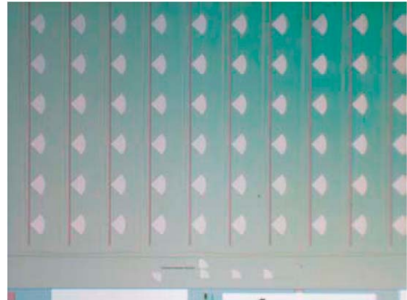
Antenna coupled focal plane prototype device Vertical lines are slots Pie shaped structures connect to the microstrip taps that cross over the slots
