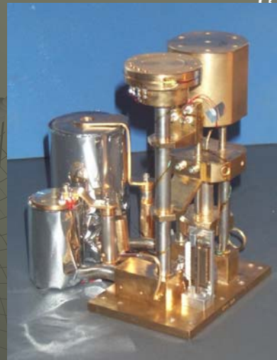
Dual stage ^3\text{He} cooler used in ZEUS/SPIFI
