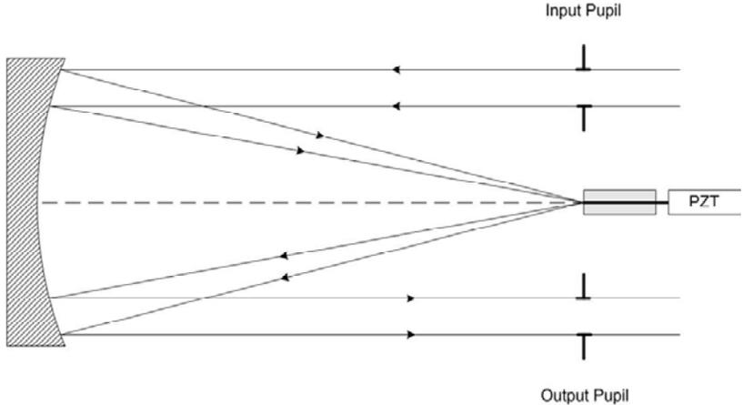
Figure 4. Cat’s eye configuration for a downstream scanning phase-contrast interferometer.
