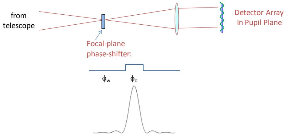
Figure 2. Layout of a transmissive phase-contrast interferometer.
