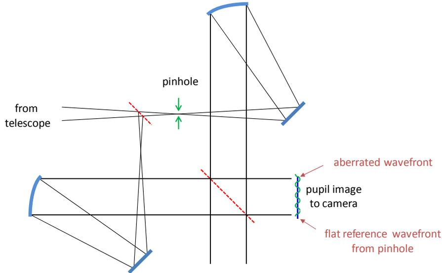
Figure 1. Layout of an all-reflective dual-beam point diffraction interferometer. Because of the physical size of the diffraction pattern, the individual optics would need to be  $\sim 30$  cm across, leading to a sizeable layout.
