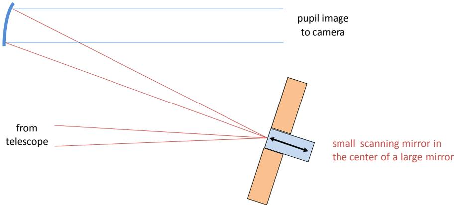
Figure 3. Layout of a reflective scanning phase-contrast interferometer. If desired, the phase shifting mirror assembly could be installed directly at the Cassegrain focus.
