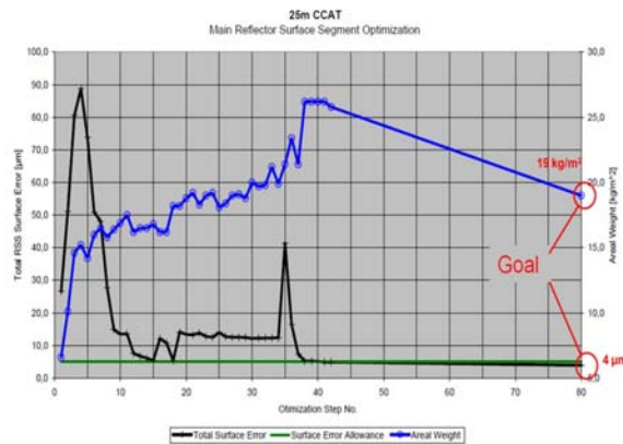
Figure 6: Vertex Antennentechnik Plot of Evolving Segment Designs vs Figure and Areal Density Goals
