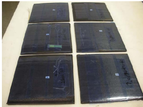
Figure 10: Unidirectional CFRP coupons fabricated for calibration/validation of composite modeling software
