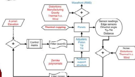
This system works very well if, as with the Keck telescopes, the panels are very stable and do not distort. The panels are the reference system for the control system, so distortions in the panels are hard to distinguish from distortions in the reflector support structure. In the best case the panel distortions effectively add random noise to the sensor readings. In a worst case the distortions are uniform across the aperture and introduce large scales distortions to the surface.
