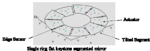
The above figure shows a simple ring of 9 keystone panels with edge sensor and actuators. A configuration for a 210 panel CCAT primary is shown below.
