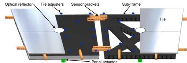
Compound panels consisting of 2 m x 2 m CFRP sub-frames and 1 m x 1 m reflector tiles. This compound panel concept separates the stiff and stable sub-frame structure from the precision reflecting tile surface.
