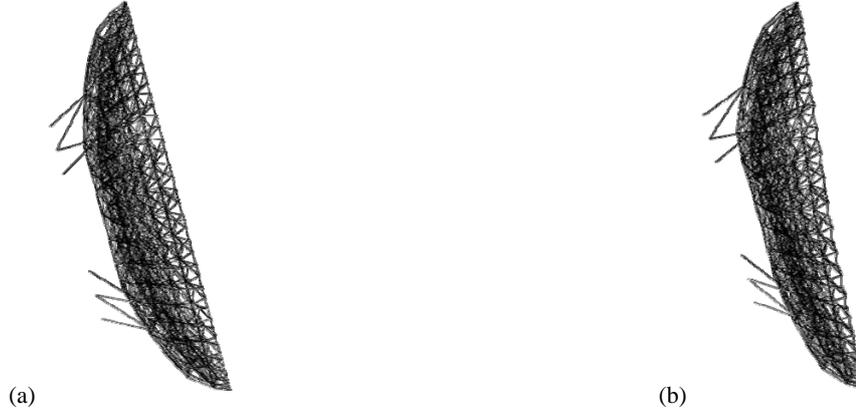
Fig. 8. Deformation due to gravity in Case 75 degree (Scheme 1) (a) Initial state (b) deformed state
