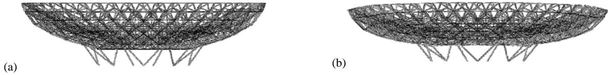
Fig. 7. Deformation due to gravity in Case 0 degree (Scheme 1) (a) Initial state (b) deformed state
