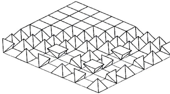
Fig.2. Composition of a slab-shaped, rectangular spatial framework consisting of semi- octahedrons and tetrahedrons
