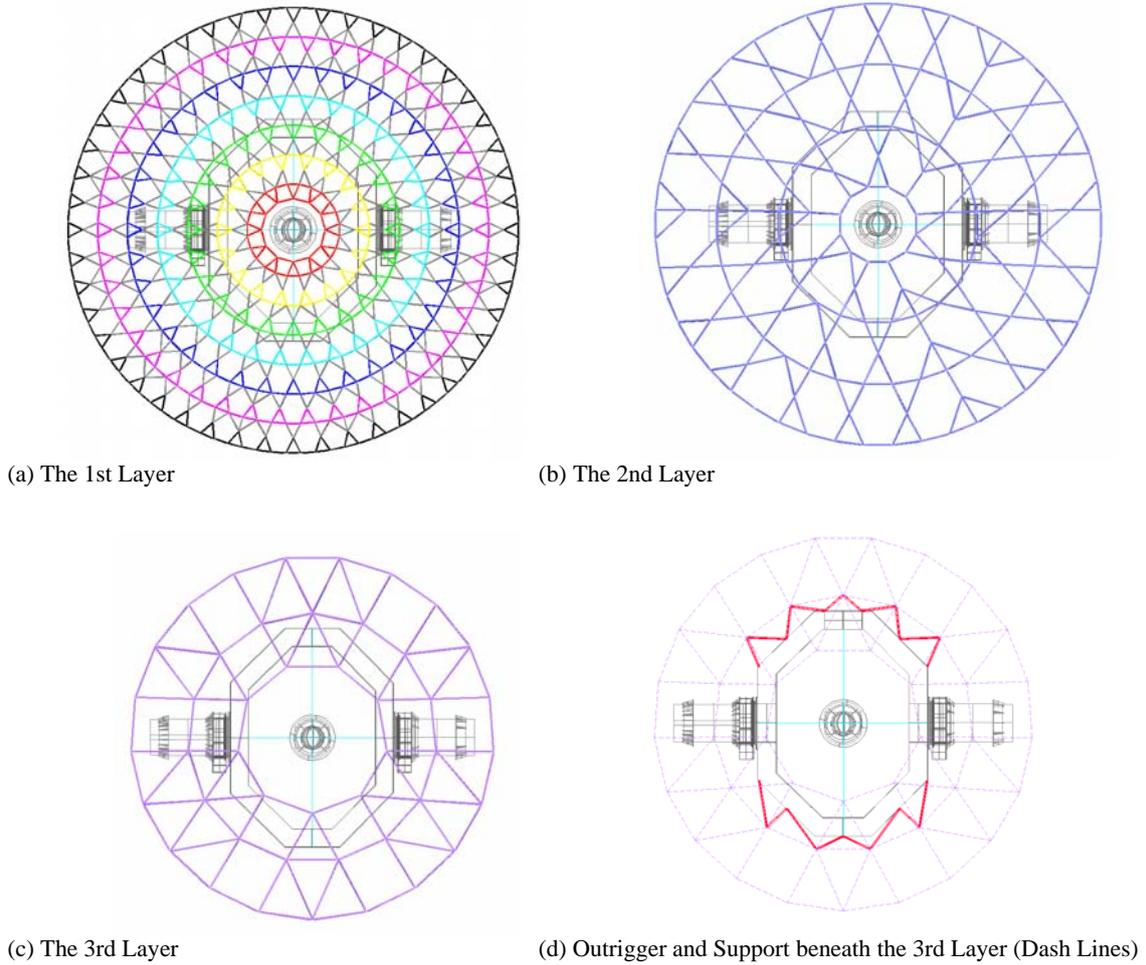
Fig. 12. Projected Plans of the Space Frame Layers (Scheme 2)
