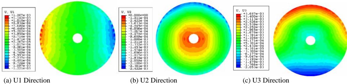
Fig. 9. Relative deformation of the 1st layer (Scheme 1)
