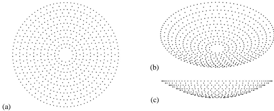
Fig. 3. Nodes of Front Surface of the Space Frame Provided by JPL: (a) Plan, (b) Bird view, (c) Elevation
