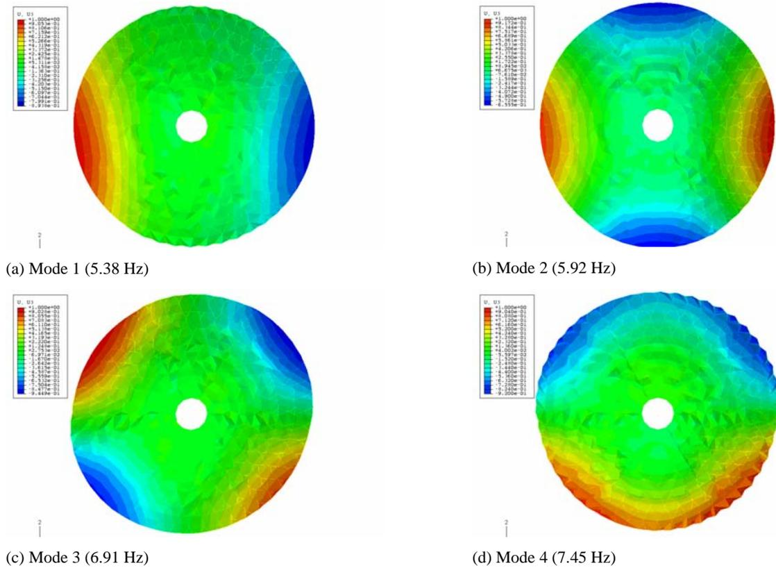
Fig. 18. Natural vibration modes and frequencies (Scheme 2)
