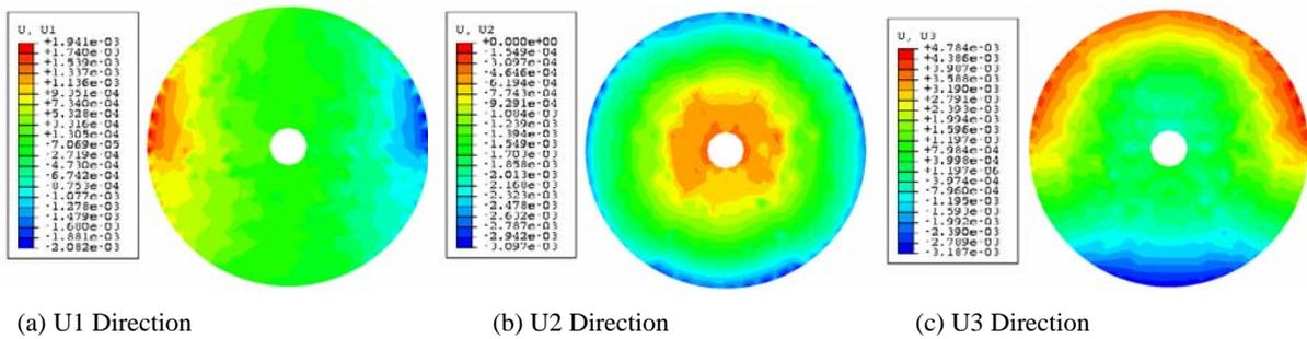
Fig. 17. Relative deformation of the 1st layer (Scheme 2)
