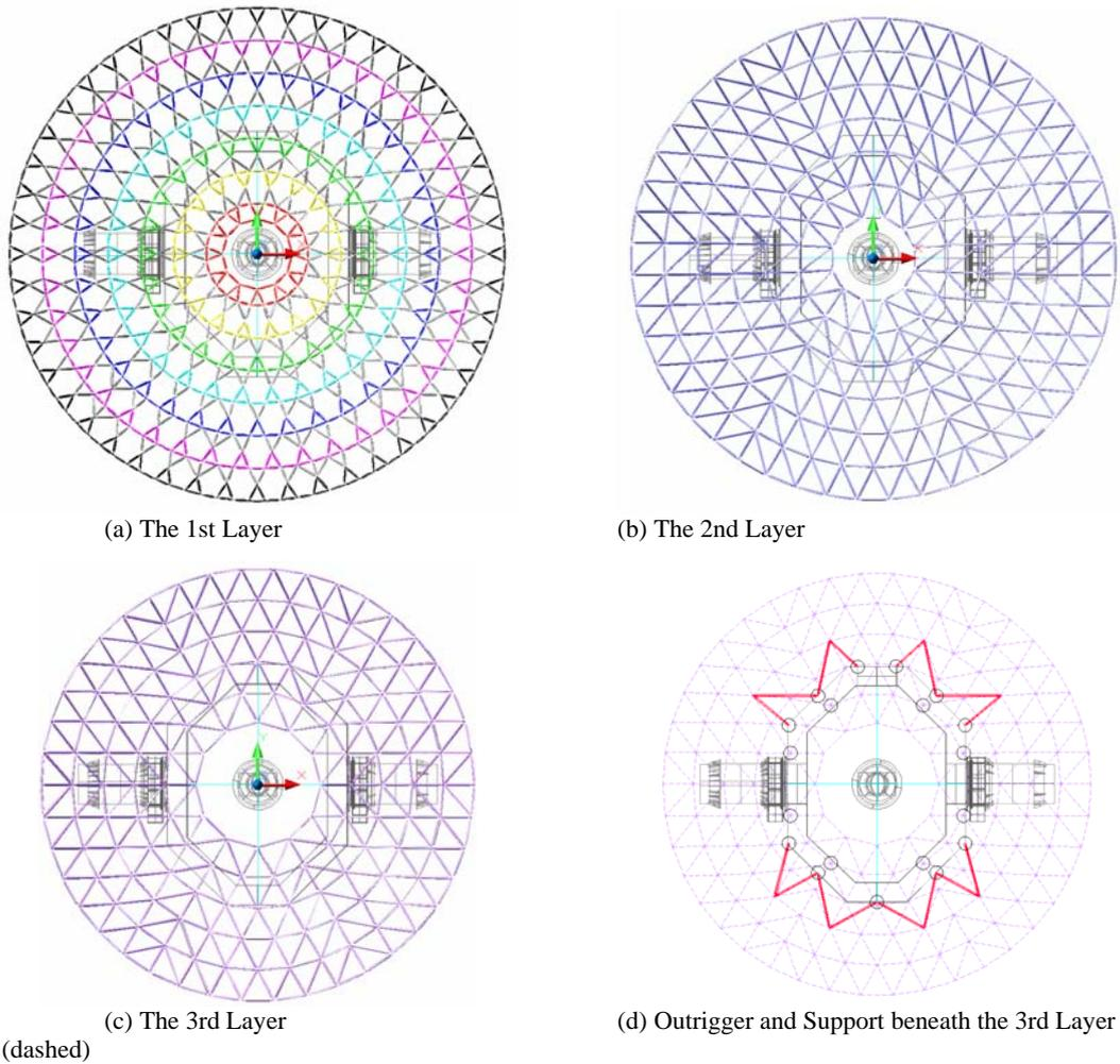
Fig. 5. Projected Plans of the Space Frame Layers (Scheme 1)
