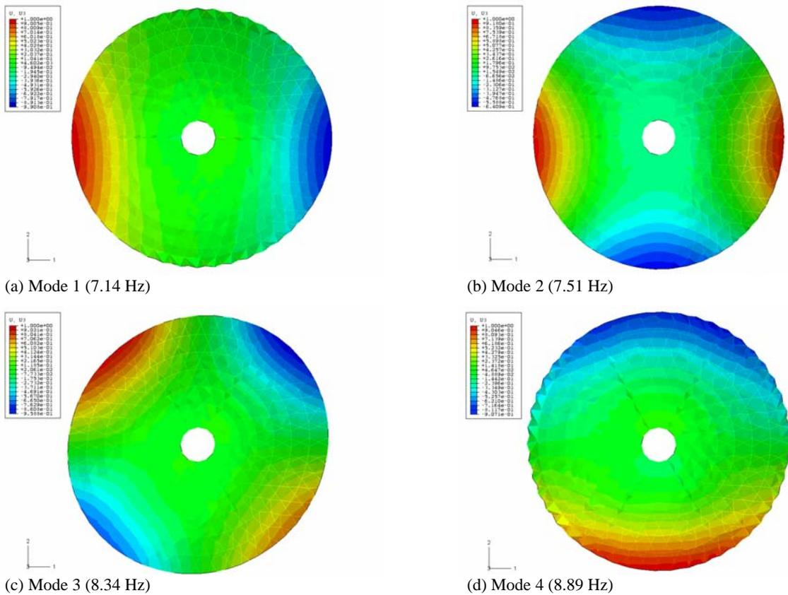
Fig. 11. Natural vibration modes and frequencies (Scheme 1)
