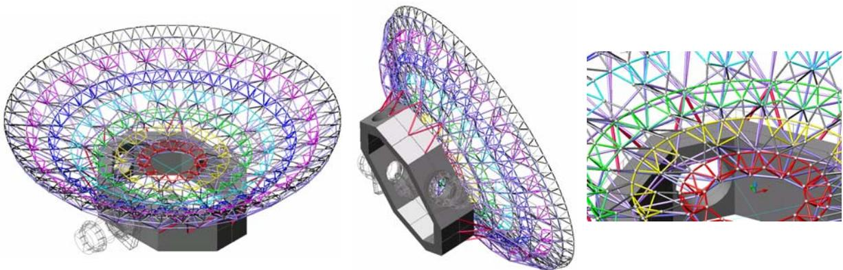
Fig. 13. Computer rendering images of primary mirror support structure (Scheme 2)
