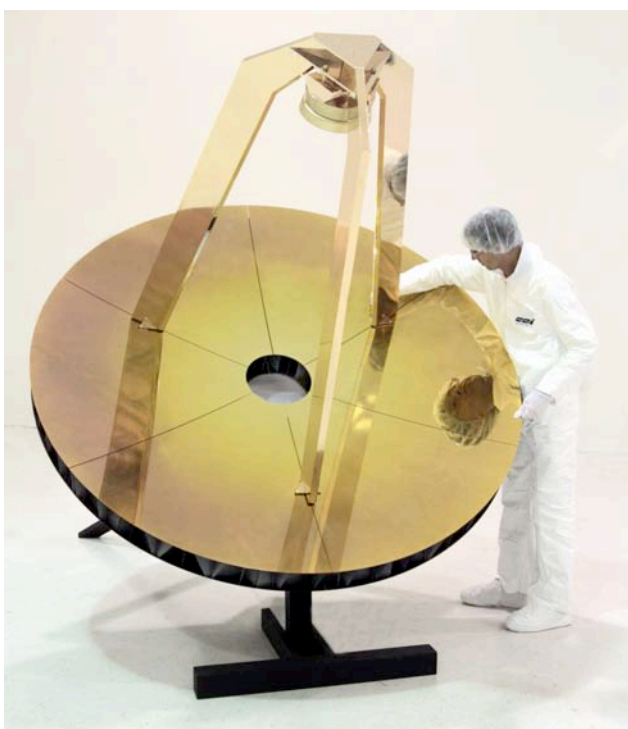
ATK Composites FIRST prototype mirror: CFRP composite mirrors of 2 meters size and micron level accuracy are within the state of the art
