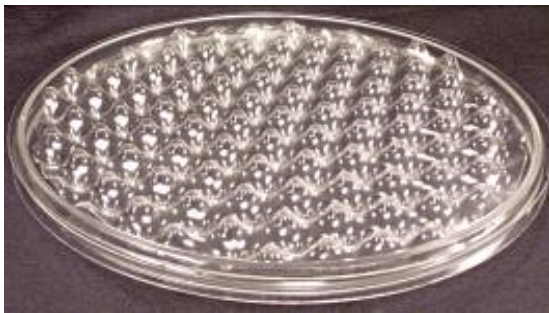
Figure 14.2.4. A corrugated mirror assembled from a corrugated core and faceplates. The assembly has high specific stiffness and thus low gravity sag.
