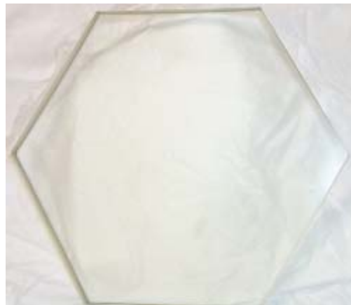
Figure 14.2.9. The 230 mm point-to-point, 19 mm thick replicated borosilicate optic. The optical surface shows considerable bubbling due to contamination during the replication process that does not show up in the interferogram because small void areas are not resolved by the interferometer.
