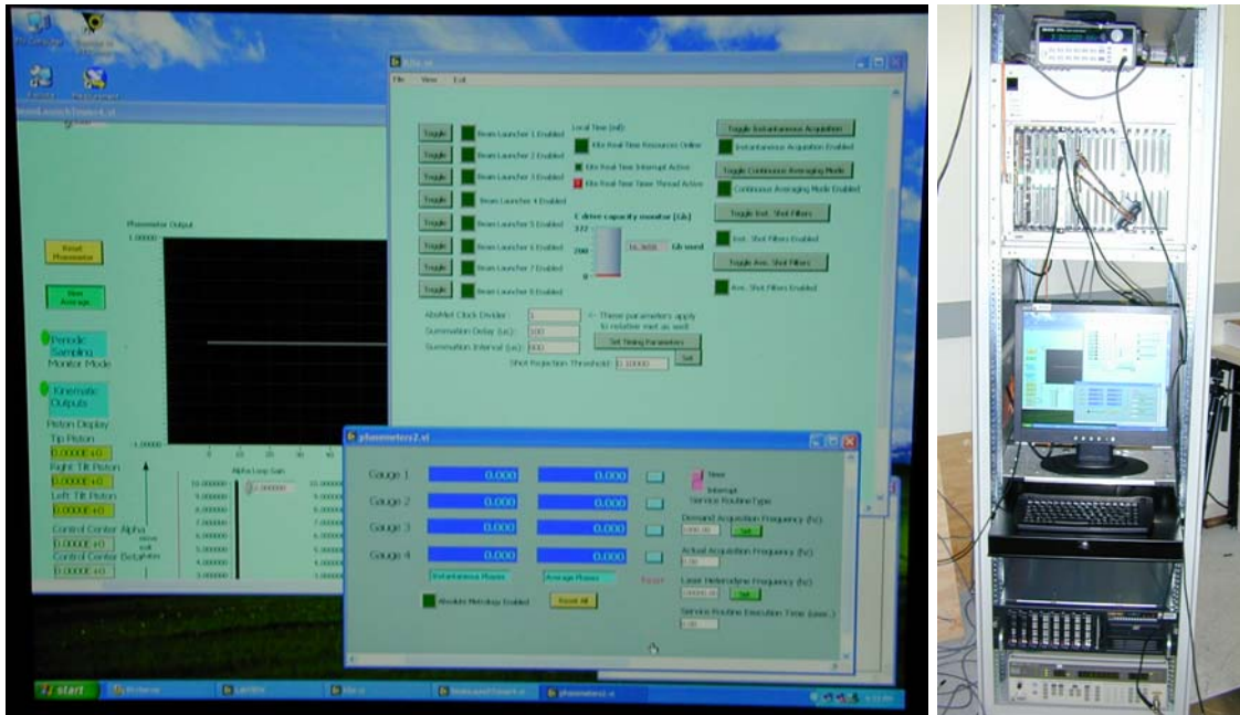
Figure 15.3.9. Left: Software interface to a CoPHI. Right: Instrument rack for testing and debugging the metrology system at JPL.
