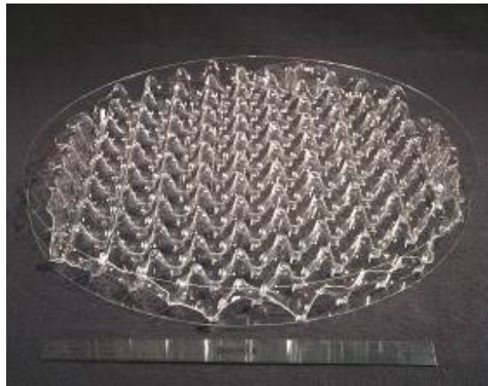
Figure 14.2.10. A half-meter borosilicate corrugated mirror blank. The ruler, included for scale, is 382 mm long.
