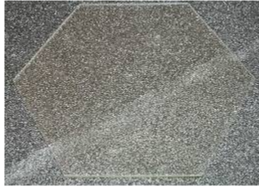
Figure 14.2.7. The 230 mm point-to-point, 3 mm thick borosilicate optic demonstrates replication of a specular surface.
