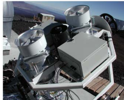
Figure 14.3.8. Two CFRP 320 mm diameter Cassegrain systems built at CMA for the ASIAA AMiBA experiment on Mauna Loa, HI.
