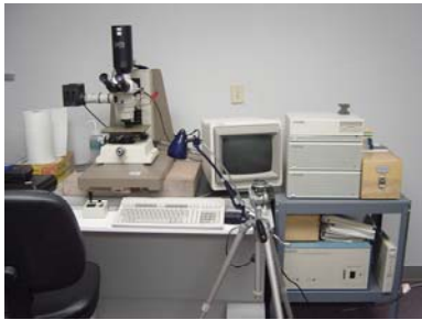
Figure 14.2.17. WYCO TOPO 3D surface profiler at CMA
