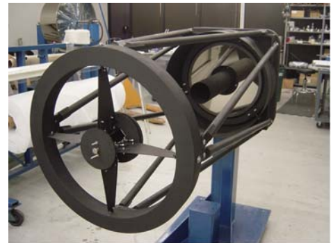
Figure 14.3.12. One of several 0.4 m optical telescopes fabricated at CMA. The mirrors and the OTA (optical tube assembly) are fabricated completely with CFRP.
