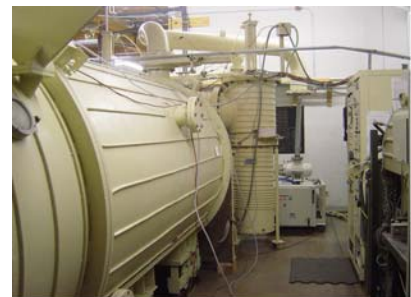
Figure 14.3.13. CMA vacuum coating chamber for large mirrors.
