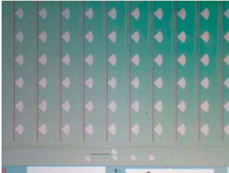
Figure 6.8. Antenna-coupled focal plane architecture prototype device. The vertical lines are slots in a niobium ground plane. Incident light with its electric field perpendicular to the slots will be absorbed. The pie slice shaped structures are connected to microstrip taps that cross over the slot; the absorbed power is directed into these taps. The power from all the taps is summed using a binary tree microstrip structure and the line is terminated with a lossy load at a power detector. The maximum wavelength to which the array is sensitive is set by the slot length and the minimum wavelength by the tap spacing along the slots and the interslot horizontal spacing. This prototype antenna used only 16 taps per slot, 16 slots, tap spacing 620\ \mu\text{m} , and slot length 9920\ \mu\text{m} , resulting in a band covering only 75-120 GHz; much larger bandwidths are possible by reducing the tap spacing (and size). The beam pattern is defined by the coherent addition of the dipole slots given the tap placement and results in a beam with a \sim 20 degree FWHM (F/2.8) at 110 GHz and first sidelobes of magnitude -13 dB at 25 deg. Beam maps are shown in Figure 10. (Figure provided by R. LeDuc (JPL).)
