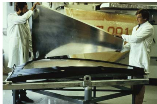
Figure 14.3.4. SMT panel and pyrex mold during fabrication at MAN Technologie
