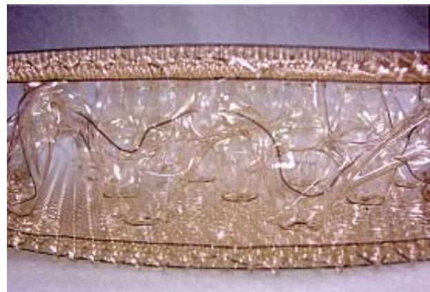
Figure 14.2.5. The additional layers in this 7-layer corrugated mirror allow a reduction of areal density, an increase in specific stiffness or an increase in the mirror robustness.
