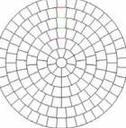
The CCAT primary mirror will be made up of multiple segments. The design shown above requires 145 panels but only six different types. This suggests the use of a replication technique which can yield substantial savings over making each panel to the requires precision.
