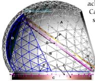
achieve full sky coverage. This Calotte" style dome is lighter, stiffer and less expensive than extrapolations of existing large telescope domes to the size required for CCAT. In addition, as both axes of motion are balances, much less powerful motors are required providing lower power consumption.
