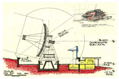
The concept design for the CCAT facility includes all necessary spaces and capabilities for operation and maintenance of the telescope and instruments. At over 5000 meters of altitude, the facility will feature oxygen enriched atmosphere within the control building to enhance operator safety and efficiency. Selection of building systems is keyed to Chilean capabilities and the logistics requirements of the high site.
