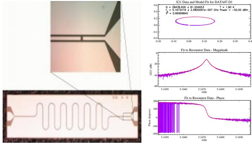
**FIGURE 2.** Left: A coplanar wave guide (CPW) resonator with gap capacitors fabricated to measure the properties of our thin superconducting films at microwave frequencies. Right: A sample fit to the complex  $S_{21}$  data from a CPW resonator.
