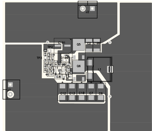
Fig. 34. Massive copper pours help spread heat.
