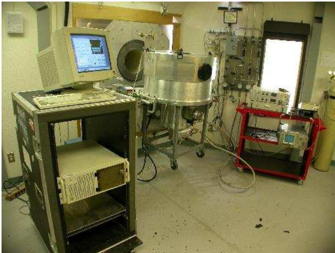
Figure 6: A picture of DesertStar mounted on the right flange of the HHT.
