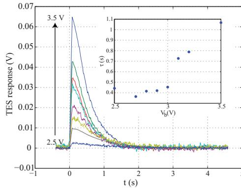
**Fig. 3** (Color online) The time response of the TES for eight different bias voltage  $V_b$  values. LED pulses were coupled into the device through a fiber optic line fed into sample box of the TES. Inset shows the effective time constant  $\tau$  for different bias voltages  $V_b$ .
