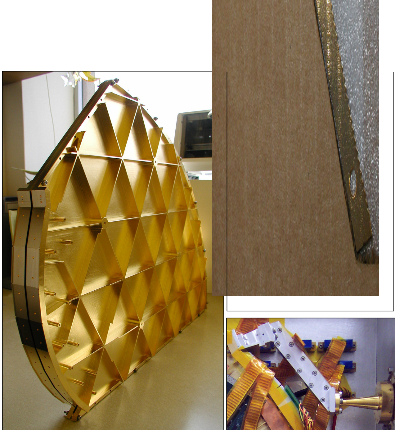
Figure 2. [Left] Z-Spec spectrometer assembled showing light-weighted rib structures. The input feed mounts on the top-most flat surface and bend blocks mount on the other eight flat surfaces. The longest dimension in the structure is 55 cm. [Top Right] View of small segment of the grating. [Bottom Right] Corrugated feed horn for coupling to the telescope, waveguide taper, and input feed which illuminates the grating.
