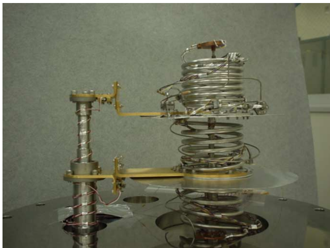
Fig. 11. Heat exchangers and cold stages (1 K, 20 K, 100 K).
