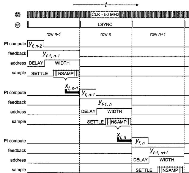
FIG. 5. Detailed timing diagram of the algorithm used for digital multiplexing.
