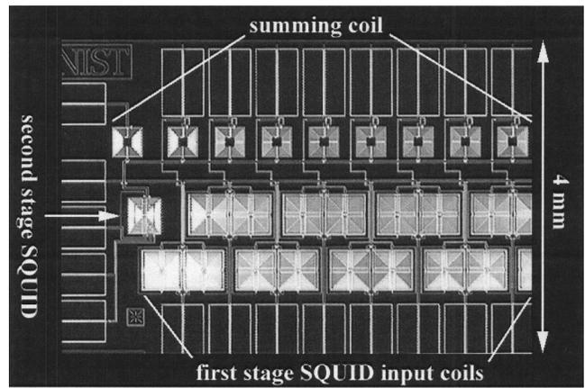
FIG. 3. Photograph of a portion of the  $1 \times 32$  channel SQUID multiplexer chip.
