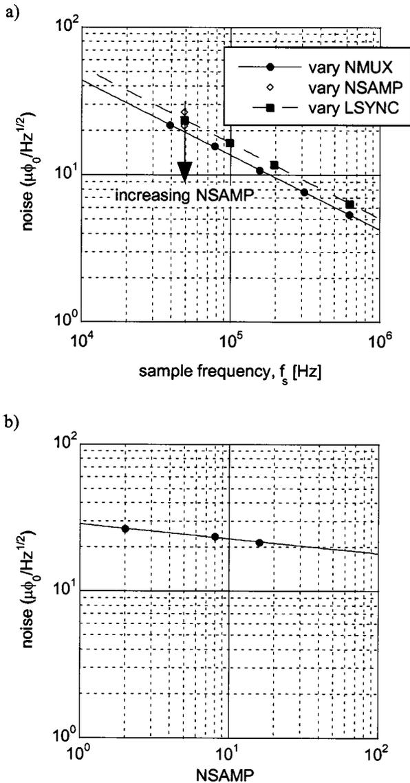
FIG. 10. Noise performance of the digital multiplexing system. Displayed in units of magnetic flux/Hz<sup>1/2</sup> as referred to the first-stage SQUID. Measurements made with an open (first-stage) input: (a) noise vs sampling frequency and (b) vs number of samples averaged during a single sampling event.
