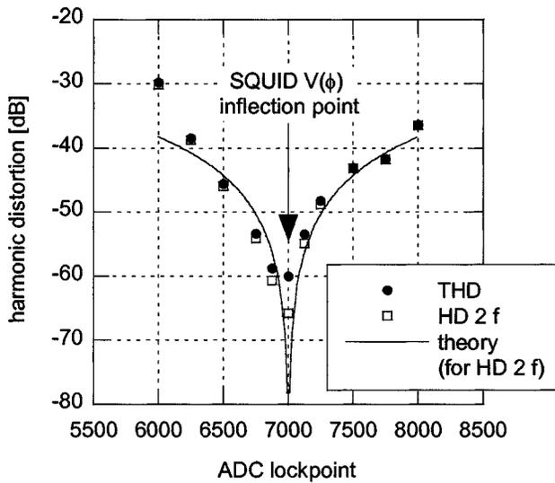
FIG. 9. Closed-loop harmonic distortion versus ADC lockpoint. A comparison to theory for a SQUID in a flux-locked loop (solid line) shows good agreement.
