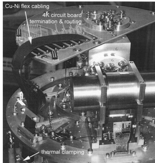
FIG. 8. Photograph of the Cu–Ni flex harness at the 4 K end (cryostat thermal shields removed).
