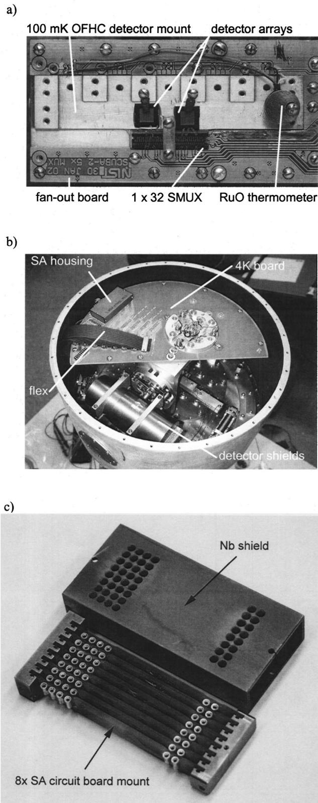
FIG. 7. Photographs of the cryostat and components: (a) a close-up photograph of the detector mount showing a  $1 \times 32$  SQUID multiplexer wire bonded to two prototype  $8 \times 8$  detector arrays, (b) 4 K working space in the cryostat, and (c) is an assembled series-array module.
