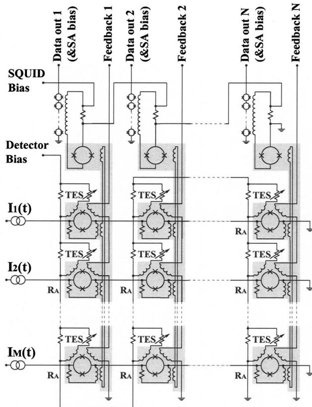
FIG. 2. Circuit schematic showing concept for two-dimensional multiplexing. Shading represents the  $1 \times 32$  SMUX chip on the detector stage at  $<100$  mK, the series array is at 4 K.
