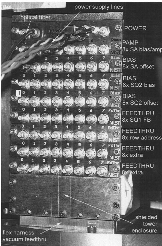
FIG. 4. Photograph of the tower enclosure atop the cryostat with analog interface electronics sufficient to operate an 8×8 array of detectors. (Cabling removed for clarity.)
