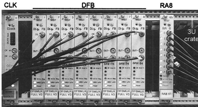
FIG. 6. Photograph of a partially filled crate of digital feedback electronics. Configuration shown is adequate for multiplexing of a  $8 \times 8$  array of detectors; eight digital feedback cards, one clock card, and one eight-channel address line driver.
