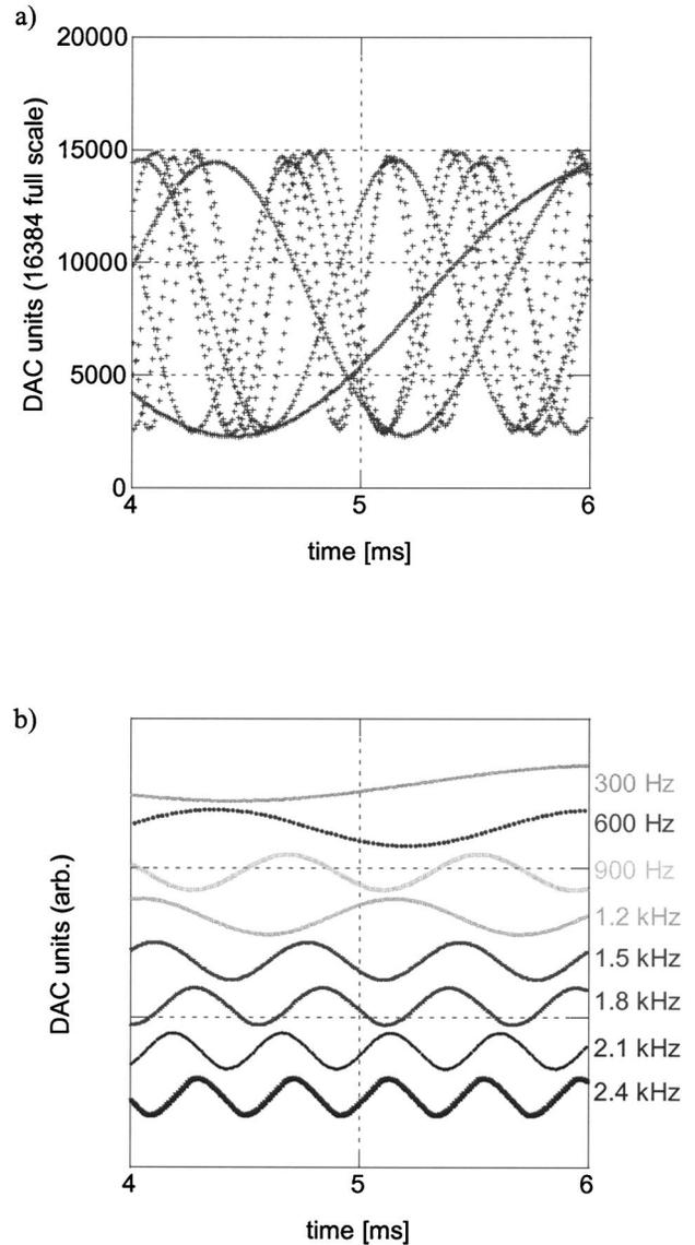
FIG. 11. Data from the multiplexing system under operation with variable frequency sine waves applied to first stage SQUID inputs: (a) real-time stream and (b) data after demultiplexing in software.
