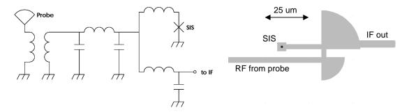
Figure 7 (left): Conceptual equivalent circuit of the RF matching network. The waveguide probe is connected to the SIS using a <sup>1</sup>/<sub>4</sub>-wave transformer followed by a lumped-element LC ladder. The capacitance associated with the SIS junction is not shown as a separate element in this figure.
