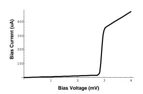
Figure 1: Modeled SIS DC IV characteristic curve for an 8.5 ohm  $R_n$  device. This characteristic curve was used throughout the mixer design process to model the SIS junction. The curve was used to generate the fully nonlinear response of the heterodyne detector model using the SuperMix software package, including predictions of mixer noise and conversion gain. The SIS IV curve depicted is typical of Nb-AlN-Nb, moderate  $J_c$  SIS junctions produced at JPL.
