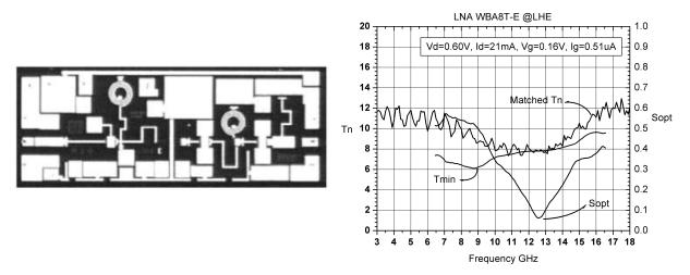
Figure 15: LNA chip and its cryogenic noise performance (measured). The WBA8T-E MMIC, manufactured by TRW, contains 4 InP HEMT stages. Using inductive feedback in the first stage to improve input match while minimizing noise, its gain exceeds 20 dB across the 6–18 GHz IF band, with a minimum noise temperature ( $T_{min}$ ) of less than 10K when the amplifier is cooled to 4K. The plot shows the measured noise temperature with a 50 ohm source ("Matched Tn") as well.
