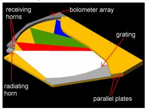
**Figure 1:** A schematic of the WaFIRS spectrometer concept shown with the top plate partially cut away. A back-to-back feedhorn receives radiation from the telescope (left) and transmits it onto the faceted grating surface (bottom). The curved grating focuses the spectrally-dispersed light onto the array of receiving feed horns and bolometers (upper left). Three beams of dispersed "colors" from the incoming "white" light are shown.
