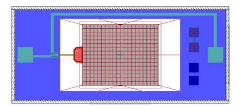
Figure 5: Z-Spec bolometer mask. The  $Si_3N_4$  absorbing mesh is in the center; the filling factor of the grid is a few percent. The square wirebond pads that are vapor deposited on the  $Si_3N_4$  top layer of the wafer can be seen on the left and right.
