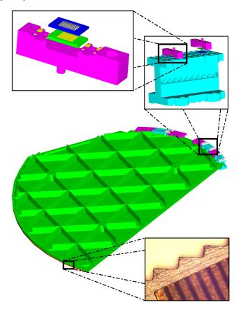
Figure 2: The grating is shown in the center with light-weighting on the exterior visible. The lower right panel is a photograph of the prototype blazed surface. Each facet (cut by wire EDM) is approximately 1 mm wide. Above and to the right is a schematic drawing of a mitred waveguide bend block. Radiation enters along the middle and is reflected up and down alternately in adjacent channels. The upper-left drawing is a single bolometer module with a backshort and bolometer shown.
