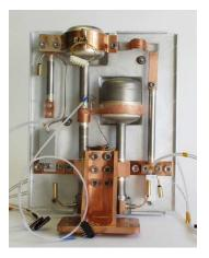
**Figure 8:** Z-Spec cryogenics. The left photo is an exterior view of the cryostat. The drum head mounting structure of the helium stage is seen in the middle. The closed-cycle <sup>3</sup>He / <sup>4</sup>He fridge is shown on the right. The pots are shown; the pumps are on the opposite side.
