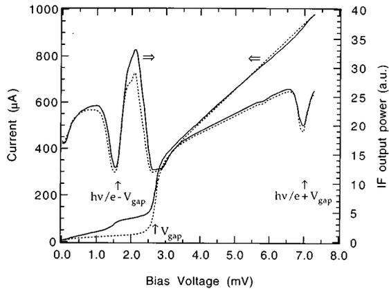
FIG. 4. Heterodyne measurement results at 4.2 K and 1042 GHz. The  $I$ - $V$  curve with (solid) and without (dashed) LO pumping are plotted, along with the IF output power when hot (295 K, solid line) and cold (80 K, dashed line) loads are placed at the receiver input. Notice that the dips in the IF power appear at the correct voltages  $h\nu/e \pm V_{\text{gap}}$ .
