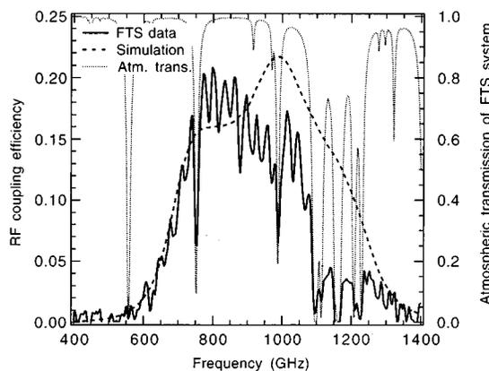
FIG. 3. Direct detection response measured with the FTS. The heavy dashed line is the calculated rf coupling efficiency. The atmospheric transmission is calculated assuming a relative humidity of 13% and a path of 3 m.
