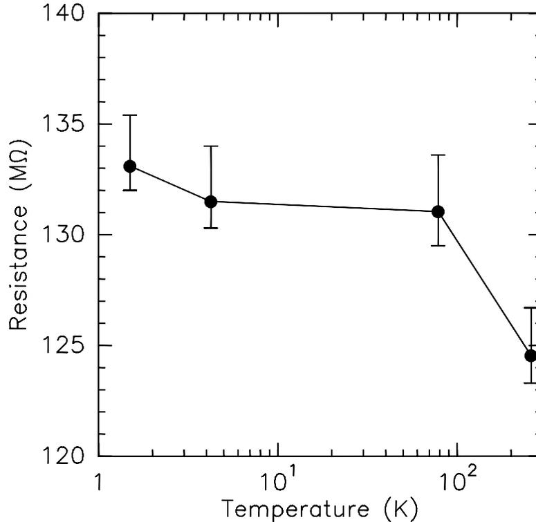
**Figure 3.** Resistance vs. temperature for CrSi load resistors in SHARC II. The resistances of a sample of 22 load resistors servicing row 6 are shown. The points show the medians, and the error bars show the 25 and 75 percentiles. The actual operating temperature is 7 K.
