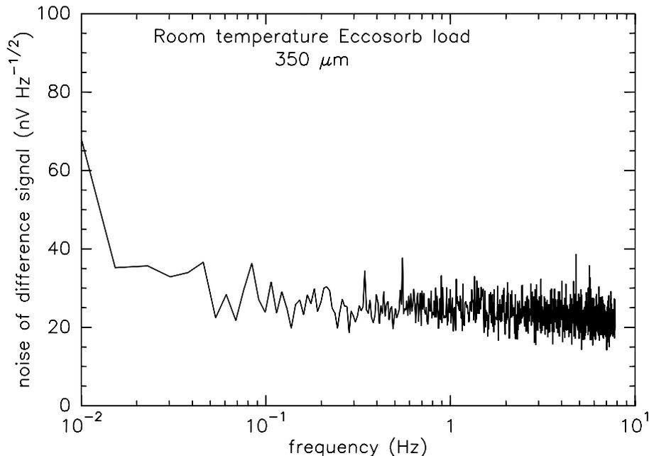
**Figure 7.** Noise spectrum for SHARC II observing room temperature Eccosorb foam. Even though shielding the foam from air currents significantly reduces correlated low-frequency noise over the array that we interpret as temperature drifts of the Eccosorb, there are still residual drifts with shielding. We show the power spectral density of the difference of two bolometer signals to subtract the residual correlated noise.
