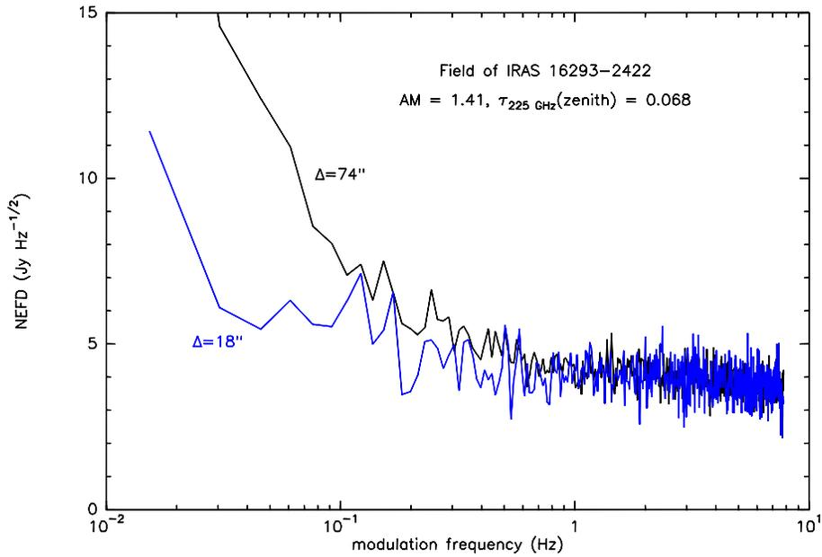
**Figure 10.** Observed NEFD for SHARC II at  $350 \mu\text{m}$  for a scanned observing mode without chopping. The  $1/f$  noise is lower for pixels separated by  $18''$  (bottom trace) than it is for pixels separated by  $74''$  (top trace), which we attribute to variable gradients in sky emission.
